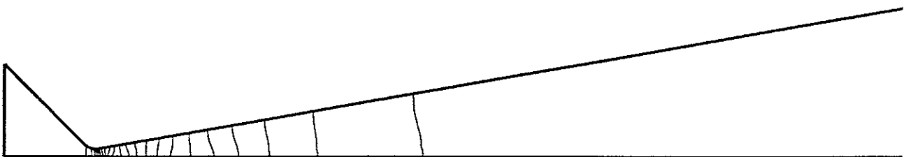
Figure 4: N_2 Vibrational Temperature. Min = 2063 K; Max = 6494 K.
