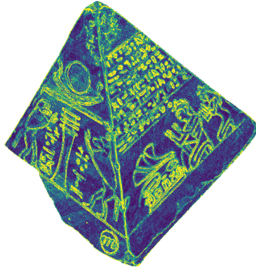
FIGURE 4. Sum of approximate absolute principal curvatures |\kappa_1| + |\kappa_2| computed at each point of a 3D point cloud from Farman Institute 3D Point Sets [DAL + 11] (colors range from blue for low values of the sum to yellow and red for high values through green). The meaningful information on the pyramid is clearly associated with high curvature values.
